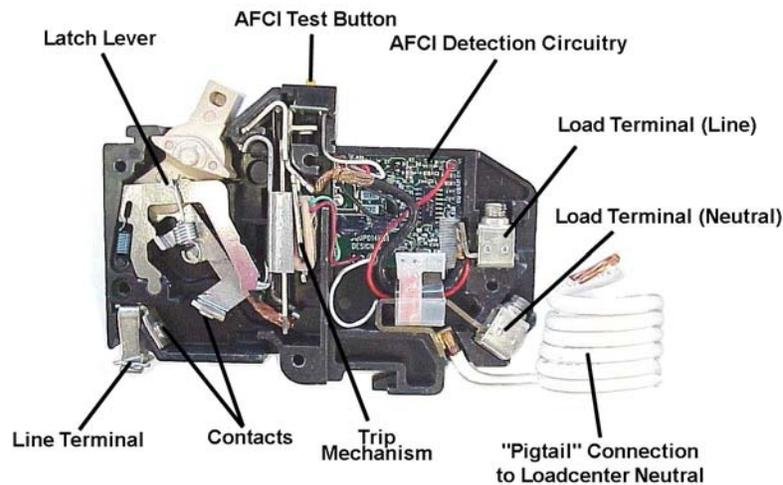
Fig. 16 – Modern AFCI Circuit Breaker
